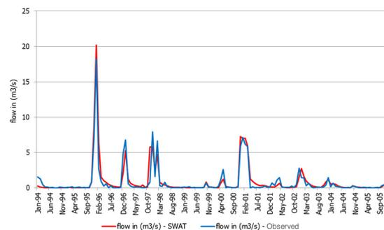
Figure 2. Model calibration for inflow to the Monte Novo reservoir
